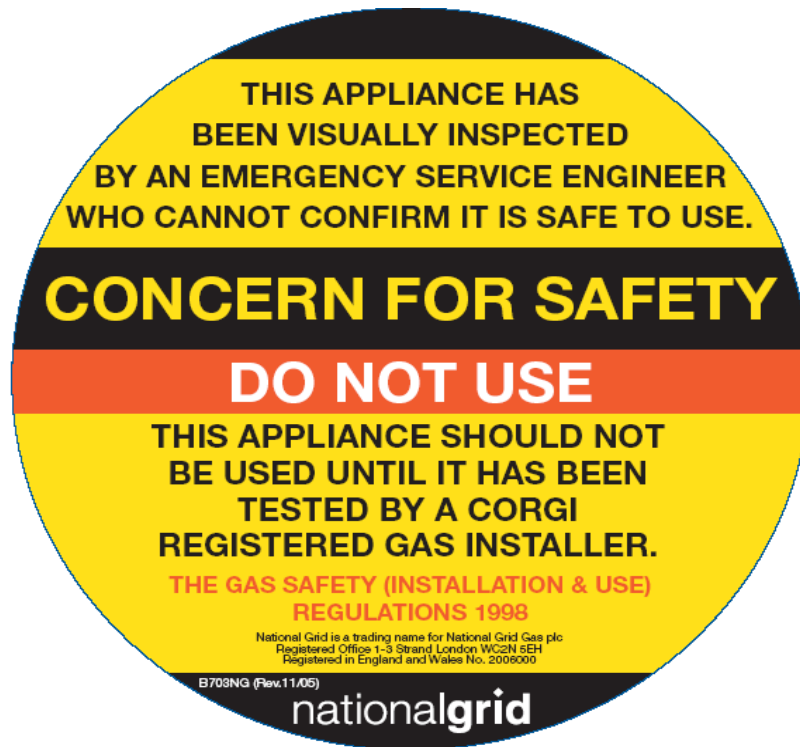
Figure 8 - Typical ESP 'Concern for Safety' label
